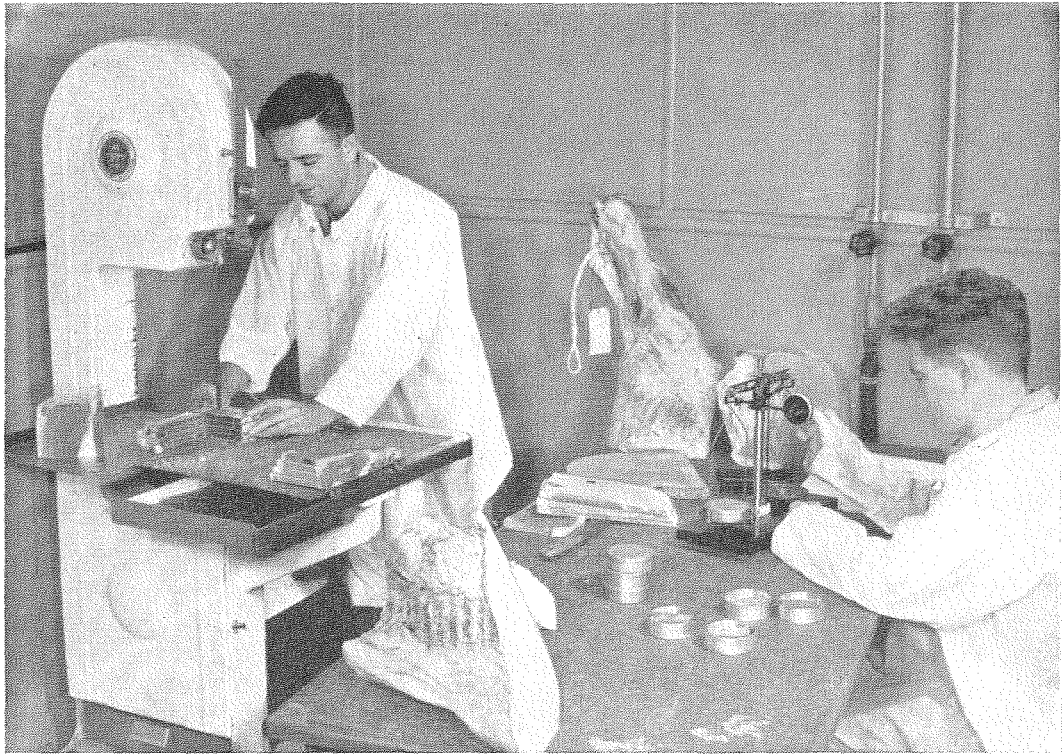
Meat Research Laboratory, Cannon Hill: Preparation of samples of frozen meat for the study of water-holding properties.
