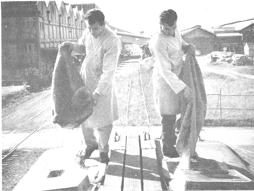
Ice being loaded into the roof bunkers of a refrigerated rail car.
