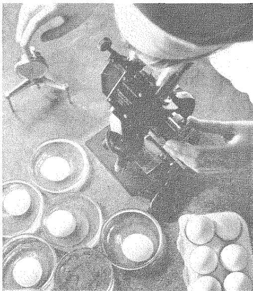
The quality of eggs may be investigated by means of the microscope and spherometer. The latter is used to measure the depth of the thick white of eggs.
