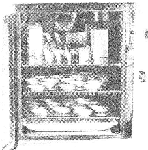
Fig. 1.—PATRA cabinet for determining WVTR under known conditions of temperature and humidity.
