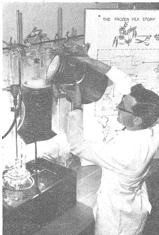
On display during the Division's recent Open Days at North Ryde was apparatus used in the various stages of a method developed by the Division for concentrating minute quantities of volatile flavours from peas (50 kg of stored, unblanched peas yields 0.5 ml of highly concentrated flavour and off-flavour essence).
