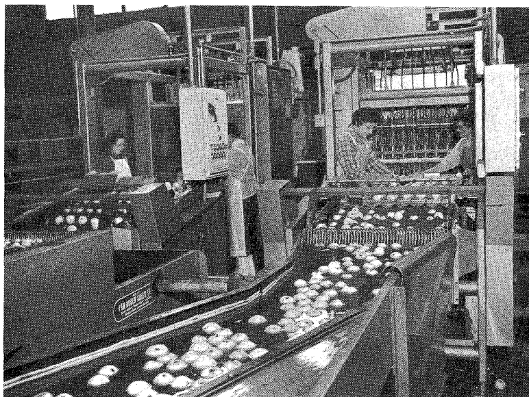
Fig. 3. — Peeled apples flumed to corer-slicer.
