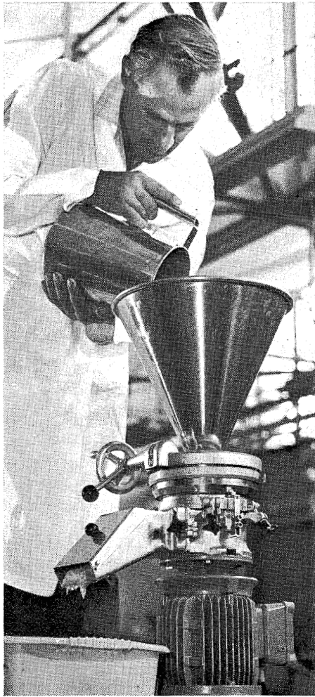
Fig. 4.—Passing the purée through a colloid mill to get rid of grittiness.
