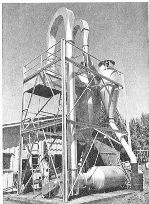
Fig. 2. Flash drier used in the last step of preparing protected lipid food supplements—drying the formaldehyde-treated oilseed homogenate.
