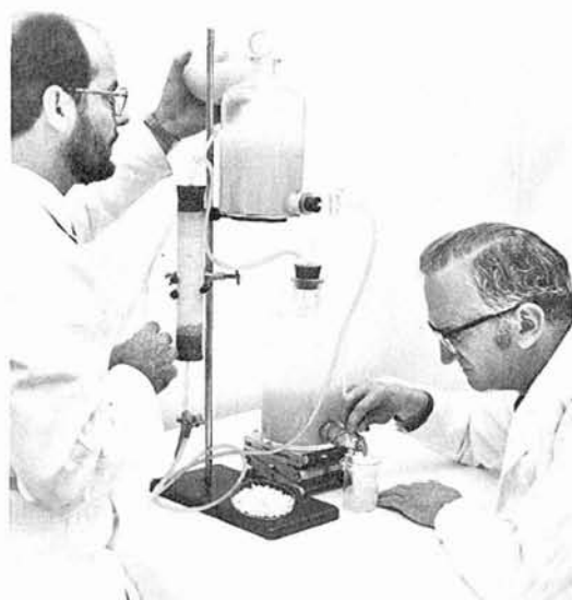
Debitting orange juice on a laboratory scale. Dr R. L. Johnson (left) is filling the juice reservoir while Dr B. V. Chandler withdraws a sample of juice for analysis after it has passed through the gel bead column. Adsorbent beads of the type used for packing are displayed at the base of the stand.
