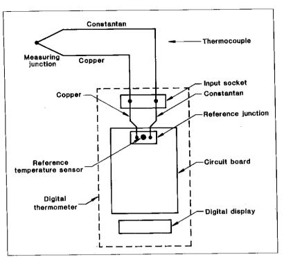
Figure 3. A Type T Thermocouple connected to the input of a digital thermometer, showing the input connector and reference junction.
