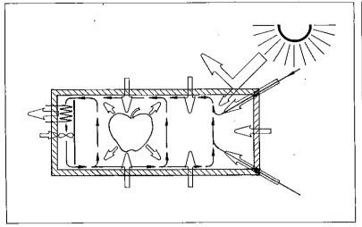
Figure 1. The container's refrigeration unit must remove heat from many sources, including the sensible heat of a stow that has not been pre-cooled, heat conducted from the walls, heat entering as airleakage and(with fruit and vegetables) the heat of respiration.
