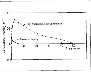
Figure 4. Transient responses of a Type K digital thermometer after transfer from a room at 22 °C to a room at 38 °C, while measuring the temperature of wet ice (0.0 °C).
