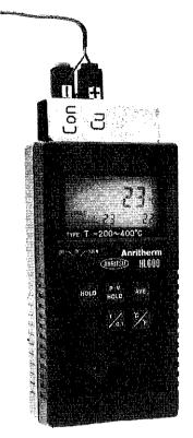
Fig. A3. Spring terminal thermo-couple adaptor fitted to digital thermometer.
