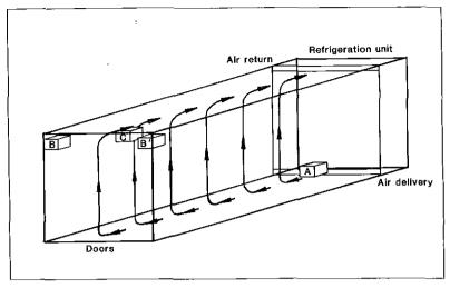
Figure 2. Locations of the coolest and the warmest parts of the stow in a bottom-delivery integral container. A: the coolest carton; B or B': the warmest carton when the wall heat load is high and C: the warmest carton when the wall heat load is low and/or the heat of respiration is high
